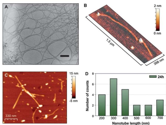
**Fig. 1** (A) TEM image of SWCNTs after 48 hours of nitric oxidation (scale bar represents 200 nm) shows high density of nanofilament entanglements, (B) typical AFM image of SWCNTs before oxidation, (C) typical AFM image of SWCNTs after oxidation for 24 hours, and (D) histogram of SWCNT lengths from SWCNTs oxidized for 24 h as obtained from AFM measurements. Note that the nanotube length is conveniently shortened under these conditions.
