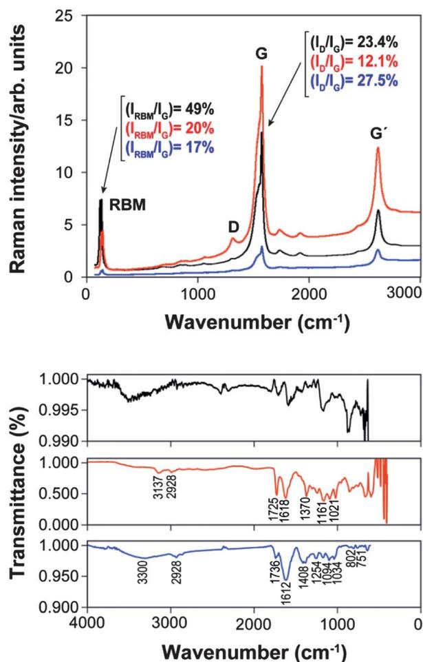
**Fig. 2** Raman (upper panel) and IR (lower panels) spectra of untreated commercial nanotubes (black) and nanotubes resulting from 24 h (red) and 48 h (blue) oxidation times.
